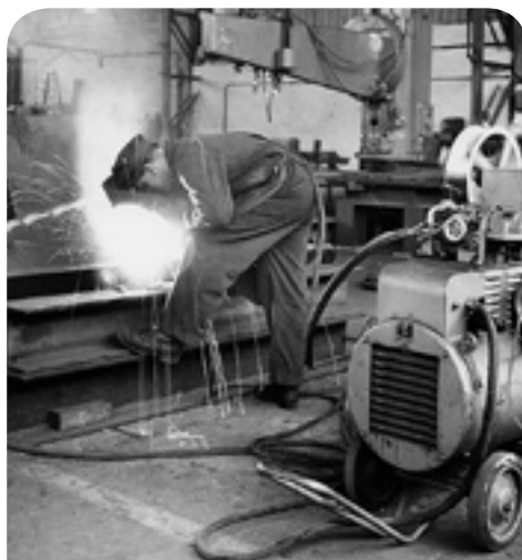
Introduction of the CO 2 gas-shielded arc welding technology by Erwin Cloos. First instance of welding using an endless wire electrode.
