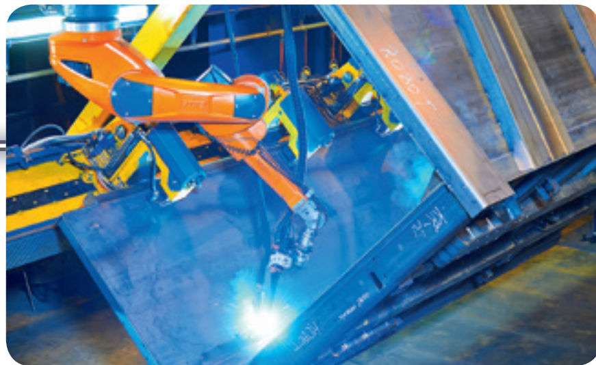
In 1996, CLOOS assumed a pioneering role with the tandem welding process. In this new process, two arcs burn in a combined molten pool.
