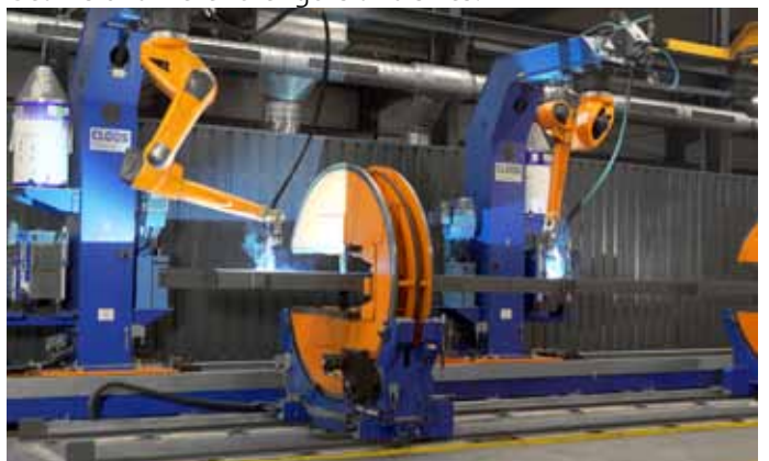
Photo 3: Mounted in an overhead position, the robots can be moved flexibly back and forth on the floor track
