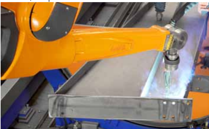
Photo 1: The QIROX robots weld complex steel components for hall production.
