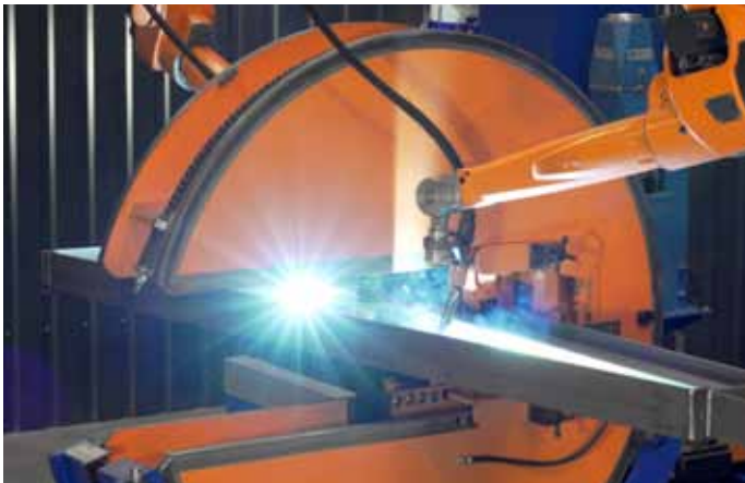
Photo 4: The workpiece positioners can support a maximum total weight of 2.5 t and can be manually moved.
